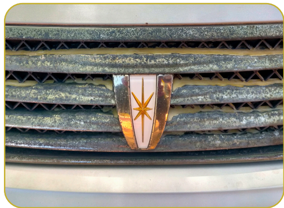
Figure 8 Accelerated corrosion on a Rotorua vehicle (Photo: Kim Smith, January 2024).
