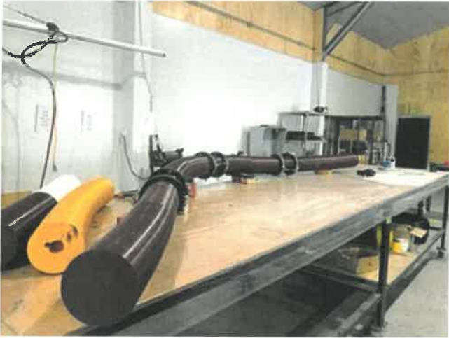
Above: gluing the 3D printed sections of the outer helix together
