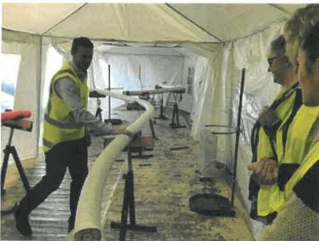
Above: sections of the inner helix waiting for layers of carbon fibre wrap
