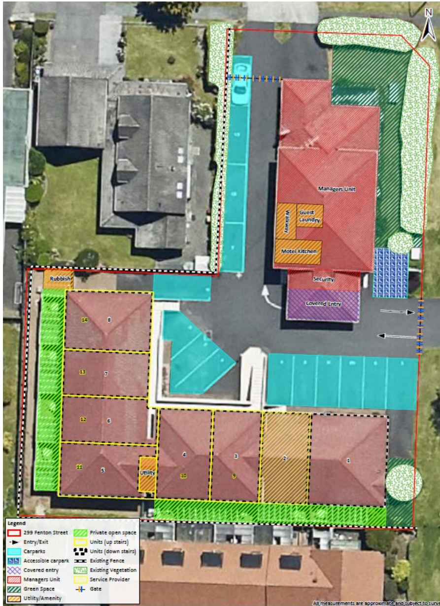
Figure 3 – Site plan showing number of units, carparking, managers unit/office and children’s play area.
